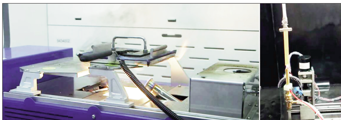
Fig. 2. Measurement of thermal protective performance on the left and vertical flammability on the right
